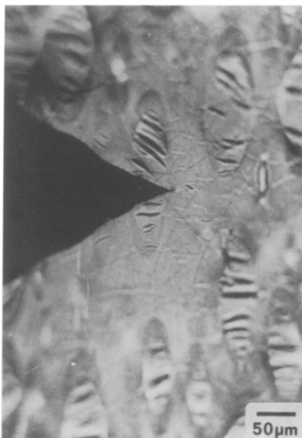
Figure 10 Growth of a diamond-shaped cavity through both matrix and polymer beads in auto-polymerized materials with 20% EGDMA (light microscopy).
