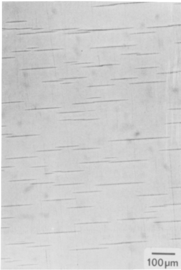
Figure 3 Crazes in heat-polymerized materials (light microscopy).
