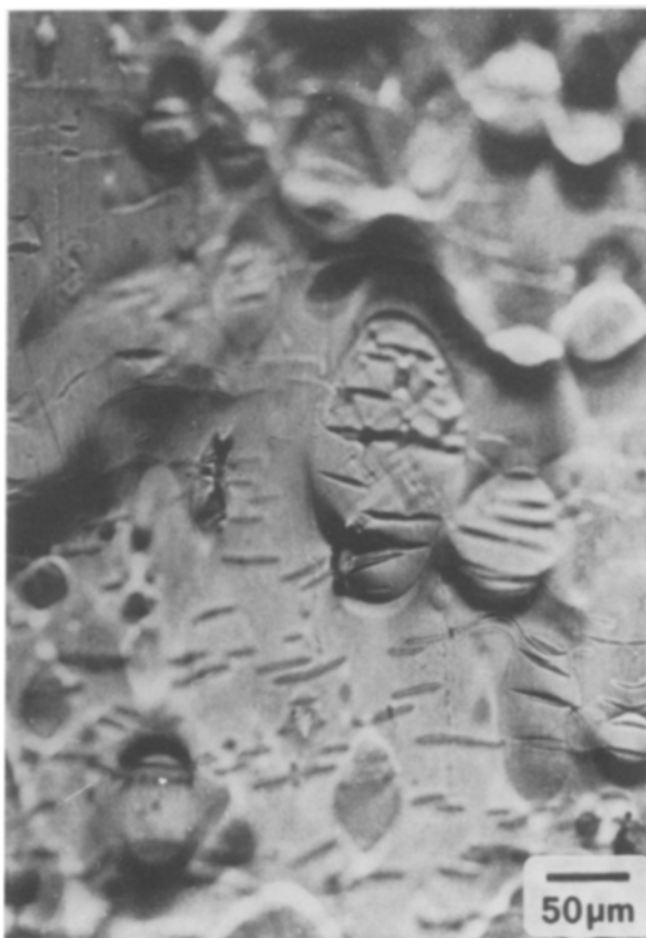
Figure 8 Opening up of a craze in the necking region in auto-polymerized materials with 20% EGDMA (light microscopy).
