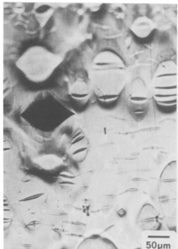
Figure 9 Formation of a diamond-shaped cavity in auto-polymerized materials with 20% EGDMA (light microscopy).
